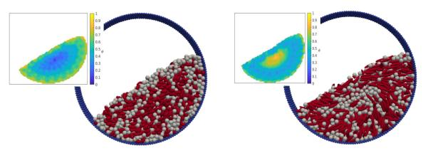
Figure 3: Mixtures of spheres and ellipsoidal particles in a rotating drum, screenshots and coarse-grained solid volume fraction of spheres. *(left)* ellipsoids of aspect ratio 2, *(right)* ellipsoids of aspect ratio 4.
