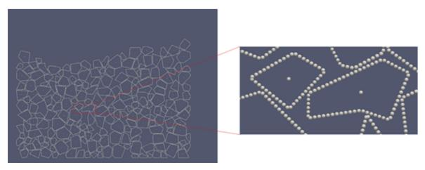
Figure 4: Multispheres reproducing the shape of ballast particles in a simulated compression test.
