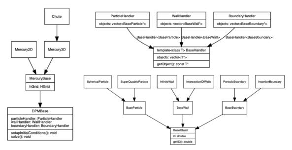
Figure 5: Basic class structure of *MercuryDPM*, showing the inheritance and encapsulation strategy. Handlers for contact laws, interactions, coarse-graining, and MPI decomposition are not shown, and only a select number of particle, wall, and boundary types are shown.
