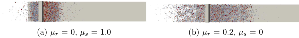
Figure 7: Top view of the spreading process at t = 0.08 s for v_T = 10 mm/s, \gamma = 0 mJ/m 2
