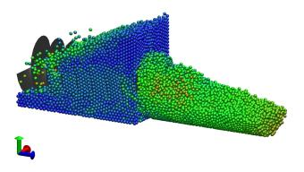
Figure 3: Snapshot of the screw feeder simulation coloured by particle velocity. The screw pushes the particles out of the box into the tube. Colours indicate particle speed. Visualisation in VMD
