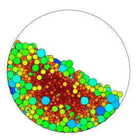
Figure 1: Poly-dispersed segregation in a rotating drum. Colour denotes particle size.
