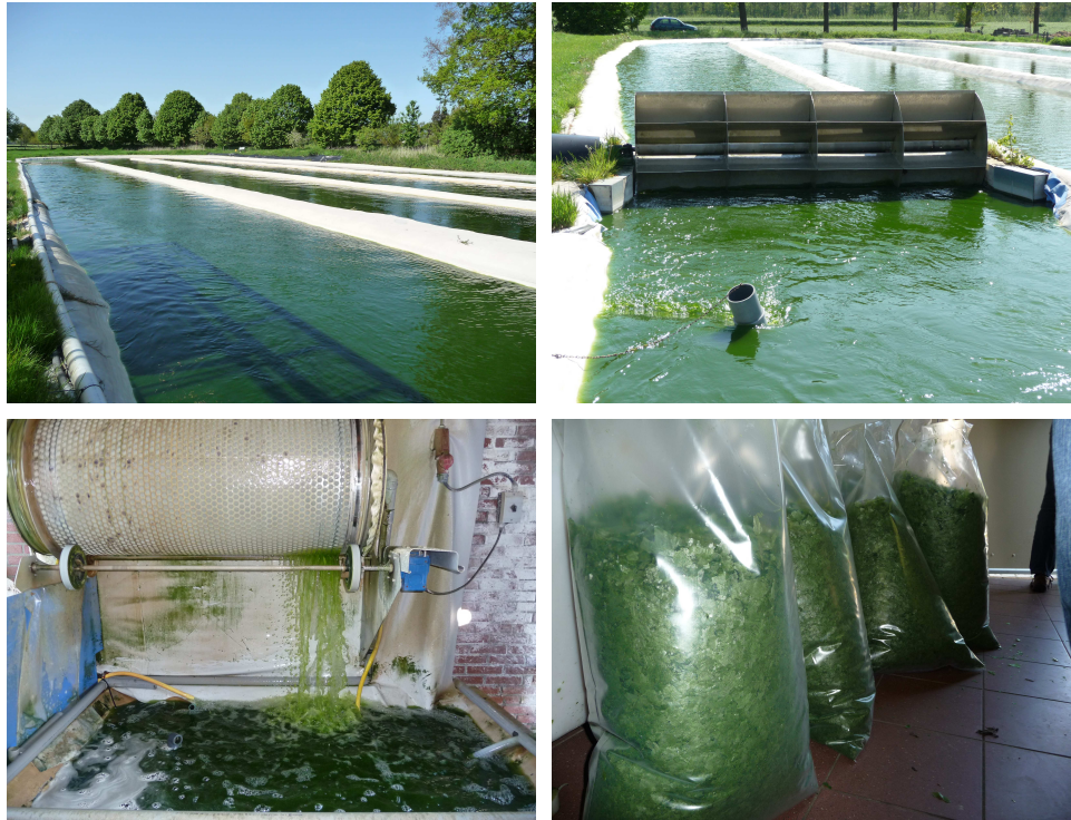
Figure 2: Images of an algae farm owned by Ingrepro: Top left, overview of the racetrack pond; top right, close up of the mixing device; bottom left, algae extraction apparatus; bottom right, bagged dry algae. Images reproduced with permission of Ingrepro, Borculo, The Netherlands. Website www.ingrepro.nl . Photos taken by V.R. Ambati.
